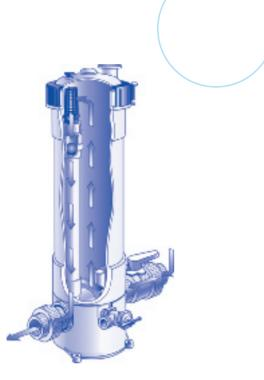
Vent valve bleeds air to ease lid removal.
