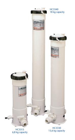
Rainbow high capacity feeders from Pentair Pool Products sanitise large residential and commercial swimming pools, using either chlorine or bromine tablets or sticks. These heavy-duty, high capacity feeders provide automatic sanitisation for pools of up to 1,260m<sup>3</sup>. They are designed for off-line hard plumbing installations using 1" PVC pipe, and are available in three sizes.
